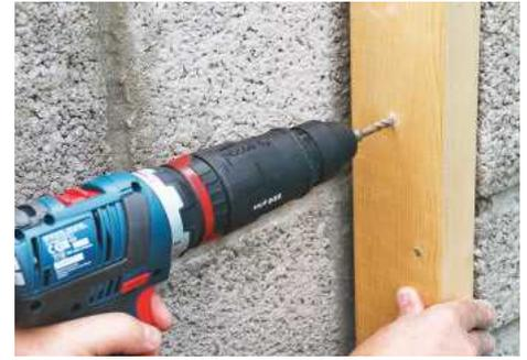
▲ The SDS chuck is powerful, quick and efficient for masonry work
